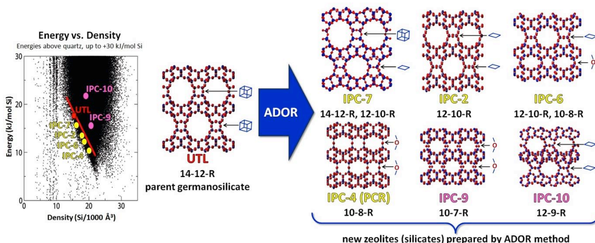
Scheme 2. The energy versus density plot (on the left) shows the distributions of thermodynamically accessible structures (black dots) and also linear fit of energy versus density for the known zeolite structures as solid red line (reprinted from Ref. [19]). The novel zeolites prepared by ADOR from parent UTL are marked on the plot as red dot for UTL, IPC-2, IPC-4, IPC-6 and IPC-7 as yellow dots and IPC-9 and IPC-10 as pink dots. Their structures with the connecting units are shown on the right.
